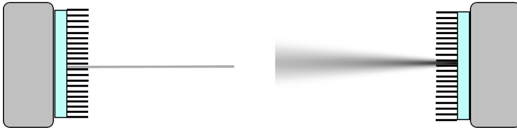
Figure 5.20: In a simple projector/backprojector, the projection is modeled as a (weighted) line integral. To account for the position dependent collimator blurring, the line integral can be replaced by a weighted integral over a cone.
