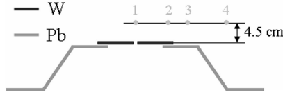
Figure 3.9: Illustration of the 4 point source locations for scatter measurement.
