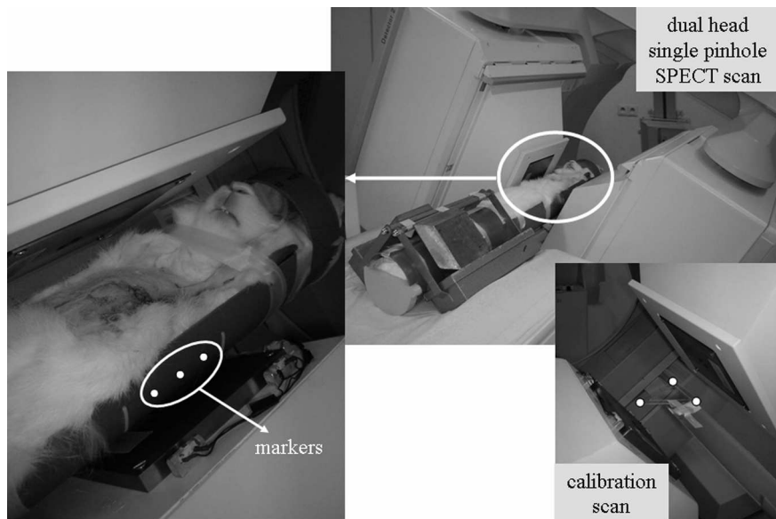
Figure 7.3: Pictures of a dual head single pinhole SPECT acquisition. The rabbit heart was positioned in the center of the FOV. Markers were attached to the rabbit bed to enable CT-SPECT registration. A calibration scan was performed immediately after the pinhole SPECT scan.
