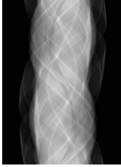
Figure 2.7: A parallel beam sinogram obtained by stacking together a number of 1D projections at different angles \theta (from 0 to 2\pi ).
